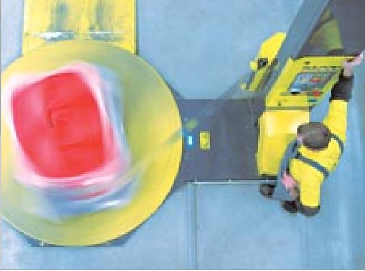
The stretch-wrapping machine automatically protects the goods and ensures safe transport.
